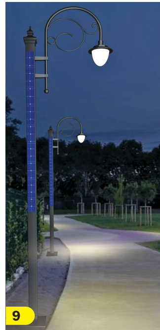
Article Code : STARCLASS (24S022/23) FRP Light Source : Led 20w/30w LED Height : 3000 mm/4150 mm Solar Pannel : Mono Perc 84w / 126w CCT : 3500k-NDL/6000k-CDL
